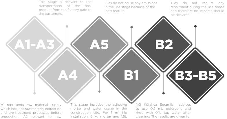
and pre-treatment processes before production. A2 relevant to raw material transportation to the plant and A3 refers to the impact occurs from manufacturing process.
