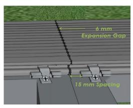
For the first board, install to the baton as detailed above. For the second board, attach a second board on a second baton/joist – as above diagram.
