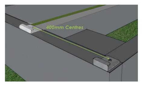
Boards should be fixed with clips on each bearer/joist. Clips should be fixed no further than 400mm apart down each side of the board. Clips should be fixed no less than 10mm in from the end of the boards (this will stop the boards falling off the clip, on contraction). Installation of hollow boards MUST use the fixing kits provided by SAiGE Longlife Decking.
